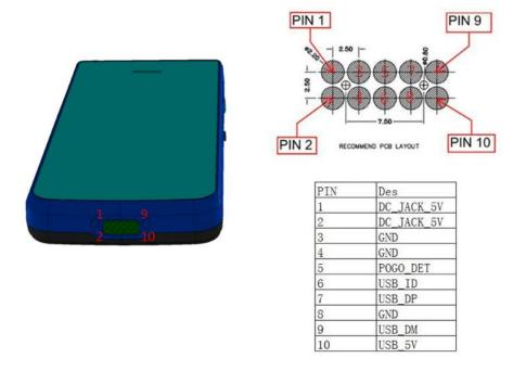
Purpose of POGO\_DET pin is to switch the USB interface from the micro USB connector to the system connector.
